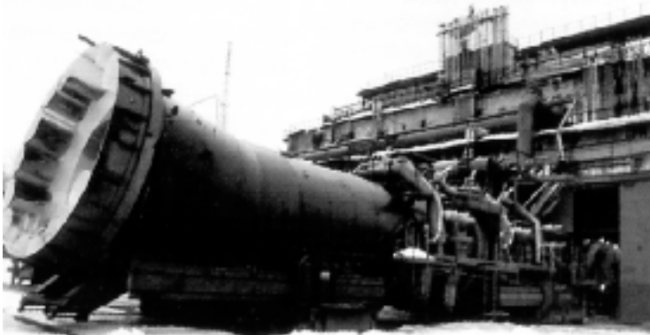
RD-0120 test stand at NIIkhimmash ( source : Russian Space Agency).
