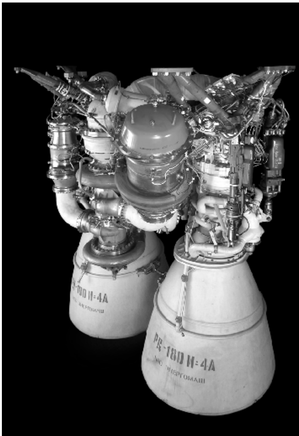
The RD-180 engine ( source : Lockheed Martin).
