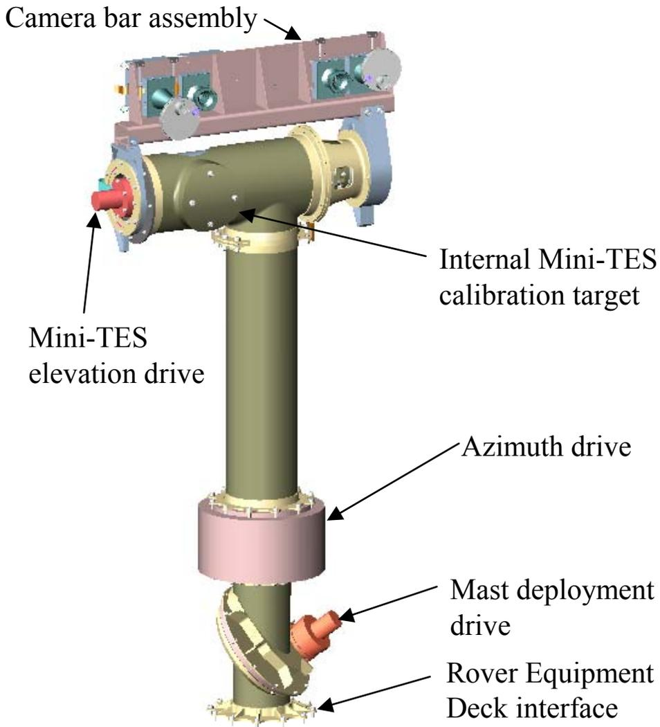
**Figure 3. Pancam Mast Assembly (PMA) configuration.**
