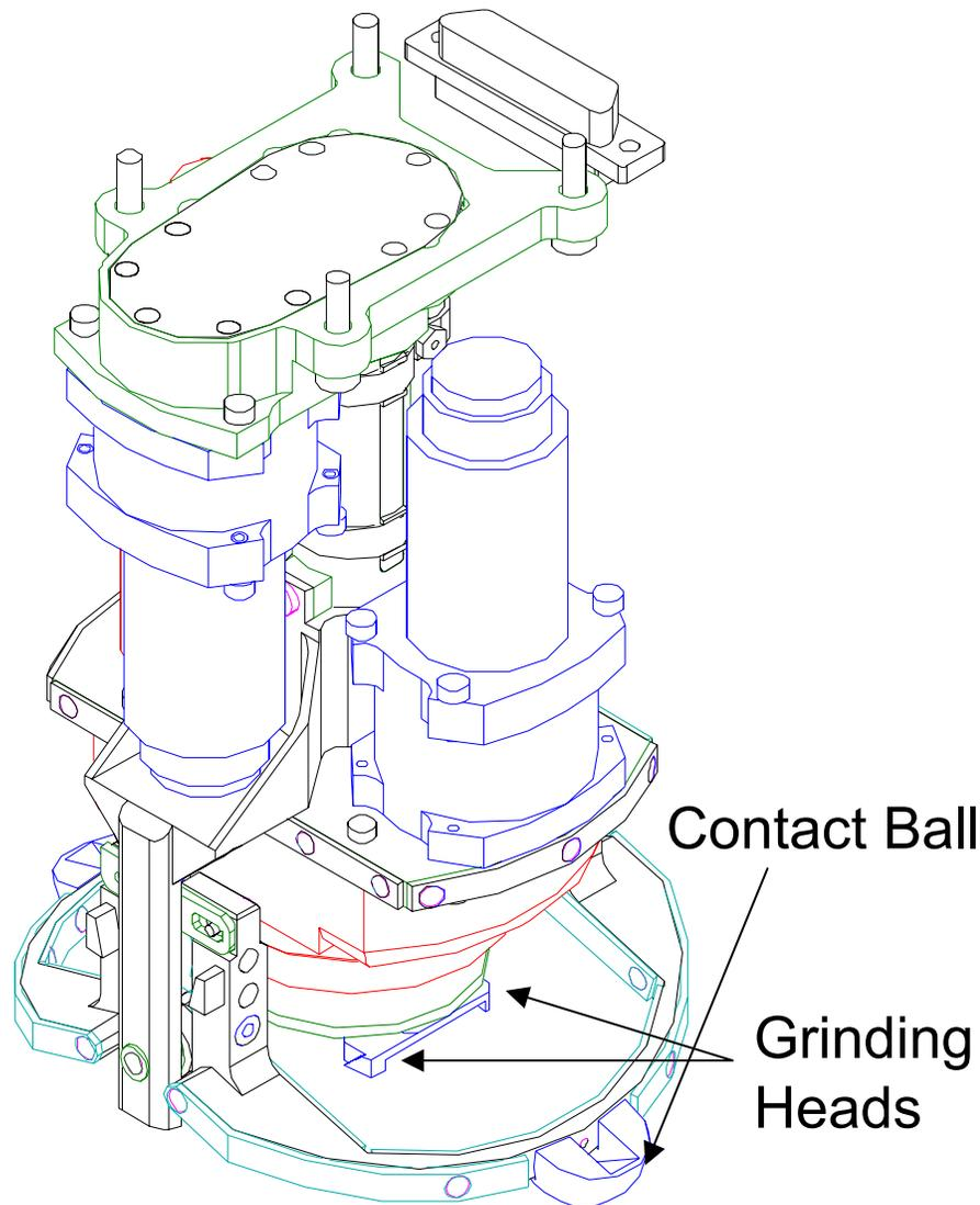
**Figure 8. Mechanical design of the Rock Abrasion Tool.**
