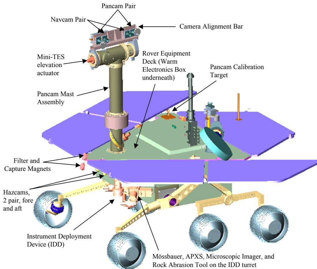
**Figure 2. Schematic diagram showing the Athena payload and cameras on the rover.**
