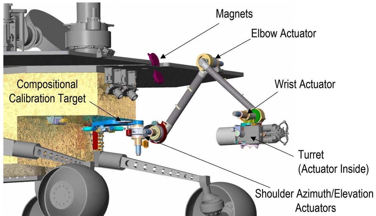
**Figure 10. Diagram showing the Instrument Deployment Device on the rover, with the payload turret on the end of the arm.**
