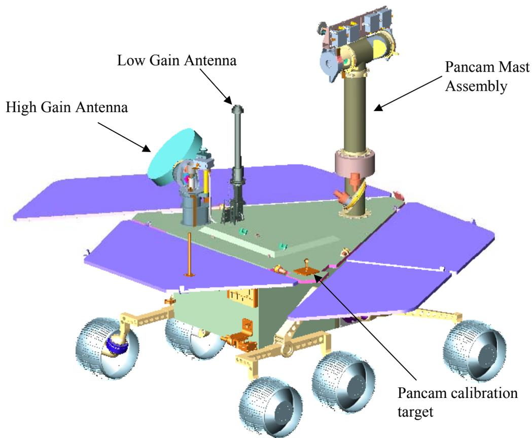
**Figure 14. Rover configuration, rear view. Deployable solar panels shown in purple.**
