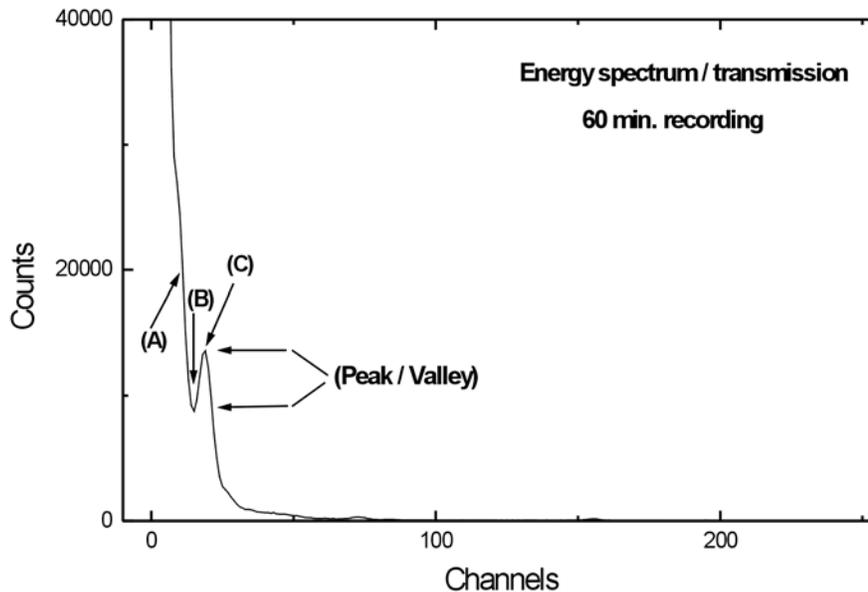
**Figure 5. Energy spectrum of a  $^{57}\text{Co}$  Mössbauer source, taken in transmission mode.**
