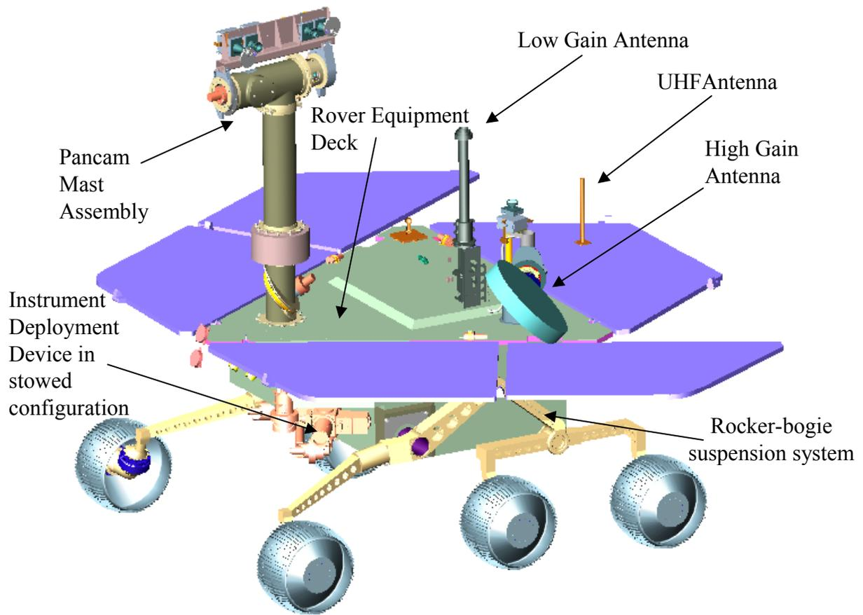
**Figure 13. Rover configuration, front view. Deployable solar panels shown in purple.**
