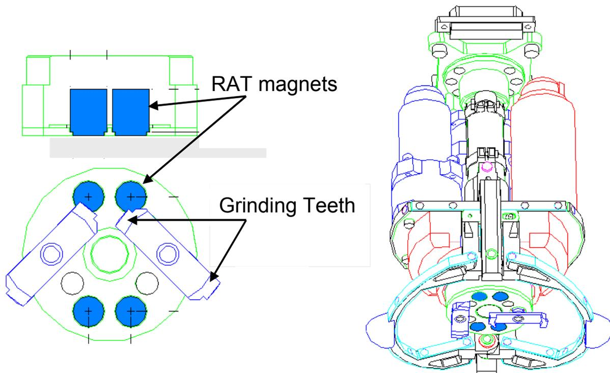
**Figure 9. Location of RAT magnets (solid blue) as seen in a view of the bottom of the RAT (lower left), in a side view of the assembly just above the grinding teeth (upper left), and in the base of the full RAT assembly (right).**
