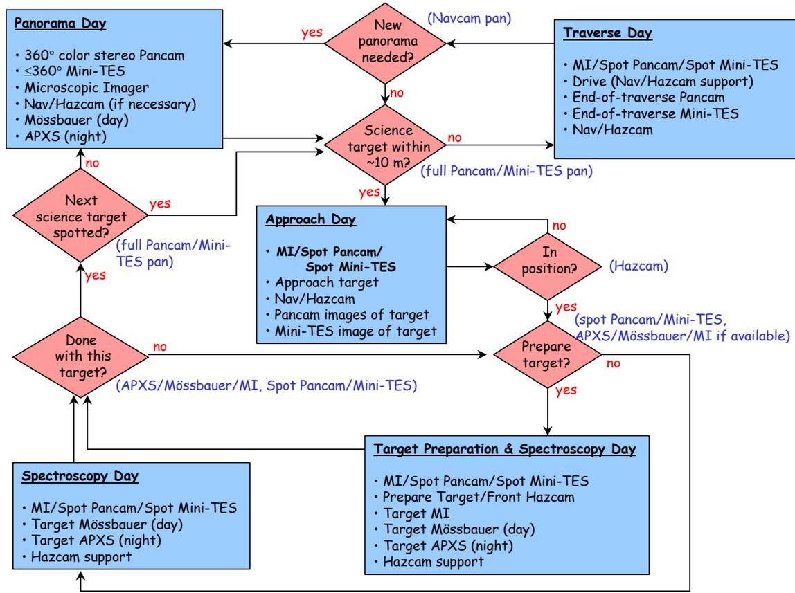
**Figure 15. MER rover operations flowchart (items in parentheses indicate data products used to make the decisions).**
