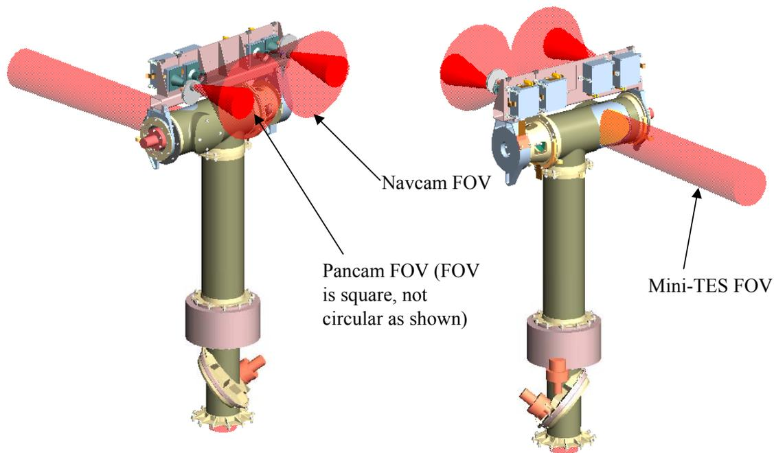
**Figure 4. Pancam, Navcam, and Mini-TES Fields of View (FOV).**
