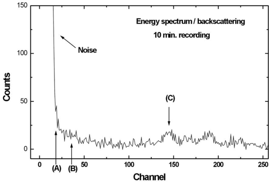
**Figure 6. Energy spectrum of a  $^{57}\text{Co}$  Mössbauer source, taken in backscattering mode on the Mössbauer calibration target.**
