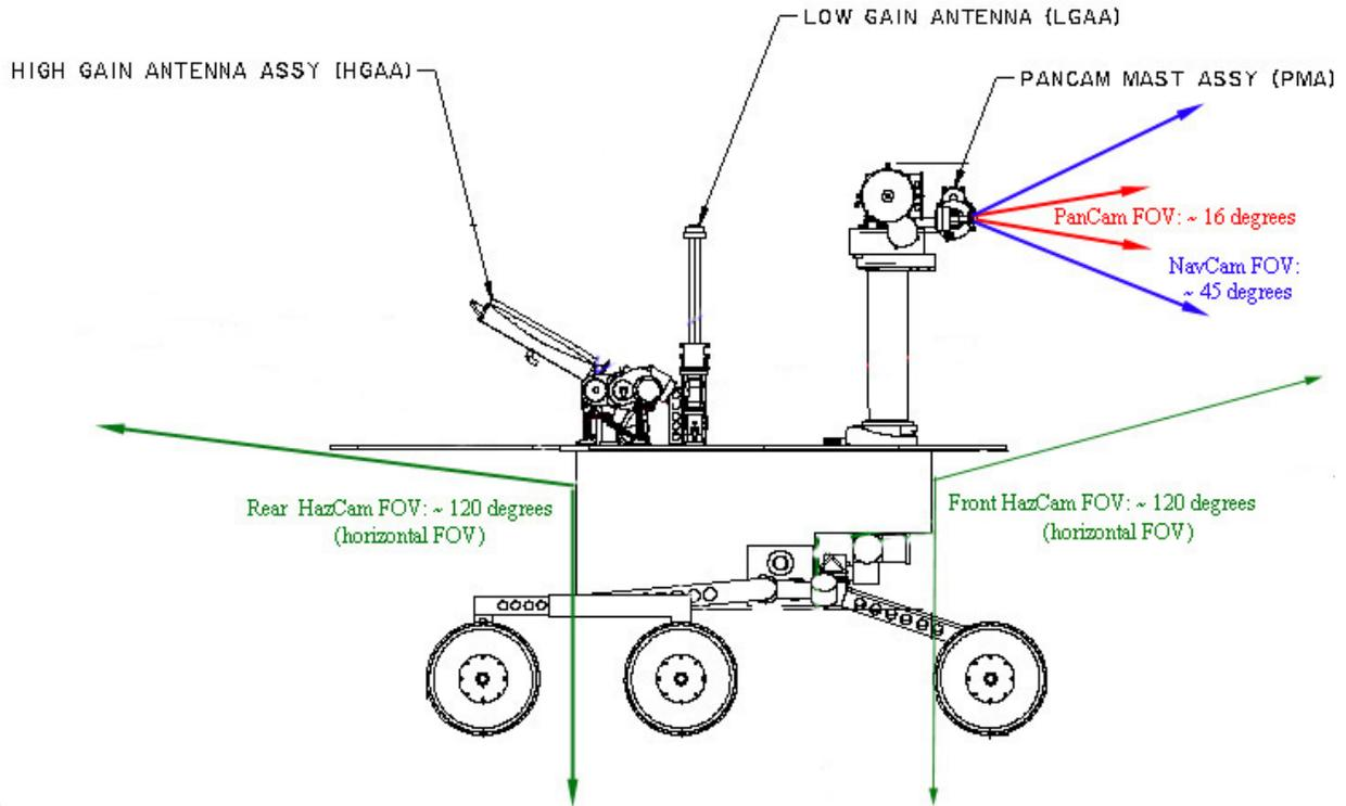
**Figure 12. Fields of view of Hazcam, Navcam, and Pancam on the rover.**
