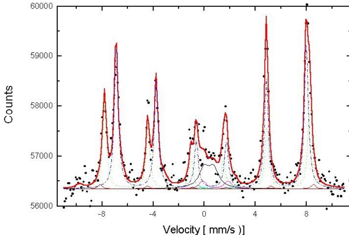
**Figure 7. Mössbauer backscattering spectrum of the Mössbauer calibration target.**
