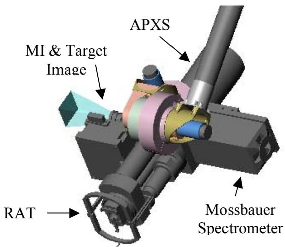
**Figure 11. Configuration of instruments and Rock Abrasion Tool (RAT) on the turret at the end of the Instrument Deployment Device.**
